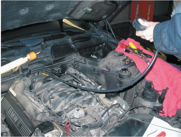
FIGURE 7 Checking the fuel pressure using a fuel-pressure gauge connected to the Schrader valve.
