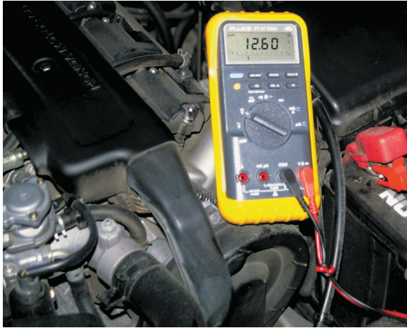
FIGURE 18 This digital multimeter set to read DC volts is being used to test the voltage of a vehicle battery. Most multimeters can also measure resistance (ohms) and current flow (amperes).
