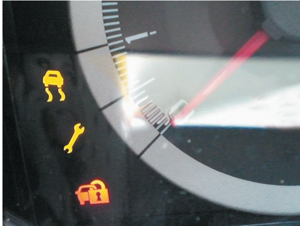
FIGURE 9 A wrench symbol warning lamp on a Ford vehicle. The symbol can also be green.
