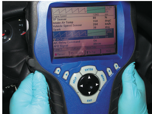
FIGURE 6 Using a scan tool to check for IAC counts or percentage as part of a diagnostic routine.
